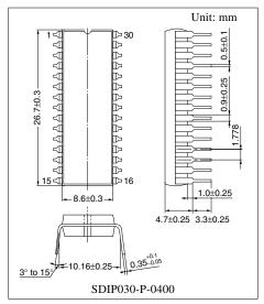
Note) The package of this product will be changed to lead-free type (SDIP030-P-0400B). See the new package dimensions section later of this datasheet.
